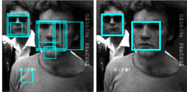
Figure 5: Left: raw classifier output. Right: detections after thresholding, merging and arbitration of overlapping detections.
