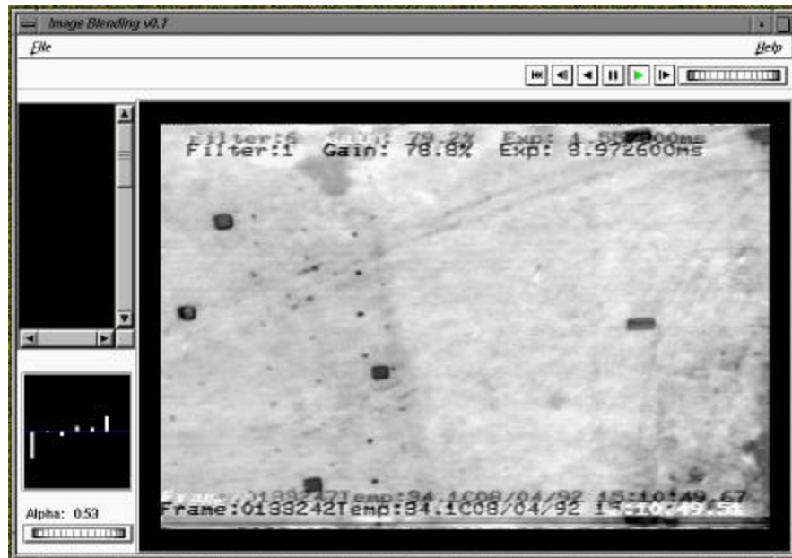
Figure 2.3: Window from the IGT minefield application. The display in the lower left hand corner gives relative intensities of contributions from each of the six filtered images.
