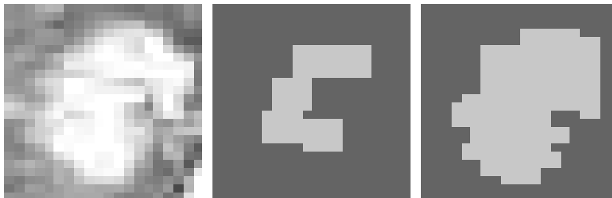
Fig. 2. Coarse-to-fine aspect of packing. Left: Sample slice (restricted to a ROI). Center: Lesion segmentation after 4 \times 4 \times 4 boxes are tested. Right: Final segmentation after 2 \times 2 \times 2 cubes and single voxels are tested, which overestimates the lesion (see section 2.4).
